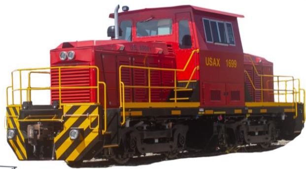
SWM9 Mid-Cab Series Switcher, Mid-mount cab 82 ton 900 hp
