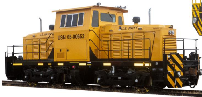
SWM9 Mid-Cab Series Switcher, Mid-mount cab 82 ton 900 hp
